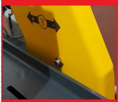
With inductive sensors located on the axes, you can use CNC without the risk of impact in axis movements
